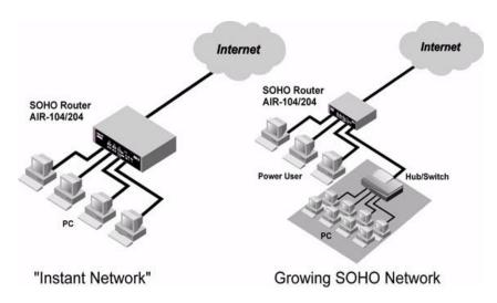
Figure 2-1 AIR-104/204 allows your LAN to expand
